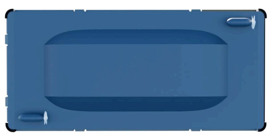
Standard OPM can be equipped with thrusters from a few hundred to a few thousand Hp in size.
